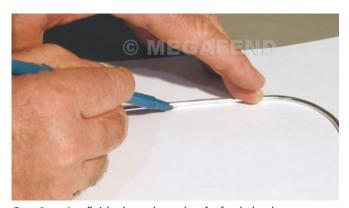
**Step 9**— Lay finished metal template for fenderhook on paper. Hold firmly in place and carefully trace pattern of inside of shape onto the paper. (A ballpoint pen is preferred for this task.)
