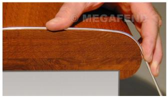
**Step 6**— While continuing to hold metal template in place flush against inboard rail side and rail top, start bend around outboard side to approximate outermost point of cap rail profile.
