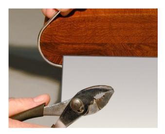
**Step 4**— Continue following contour using pliers as aid in bending rod to assure snug fit.
