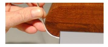
**Step 3**— Carefully bend the metal rod or strip to accurately follow the contour of the cap rail.
