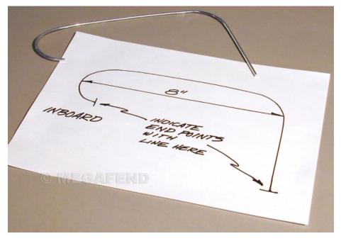
Step 10— Carefully mark ends of inboard and outboard sides of fender hook with perpendicular lines as shown. Accurately measure inside dimension (I.D.) between inboard and outboard sides of cap rail and mark on pattern. (This measurement is critical so that we can adjust the size of photo copies ar favor sent to us to match the actual size of your metal template.) Mark inboard side on pattern. When building your fenderhooks, we will make the proper allowance for sheep's wool liner.
