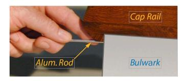
**Step 2**— Start template shape tightly flush to inboard side of bulwark where the cap rail joins.
